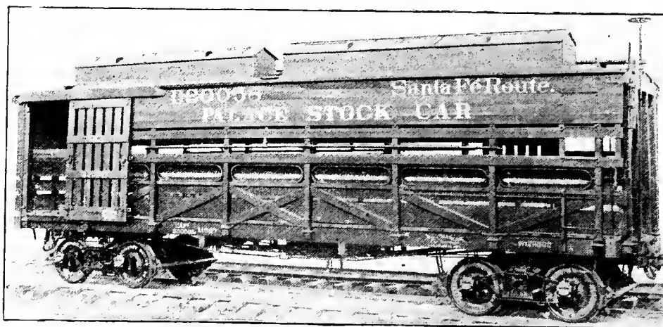
Fig. 41. STOCK CAR FOR CATTLE AND HORSES. ATCHISON, TOPEKA, & SANTA FE RAILROAD. Length, 34 ft. Capacity, 50,000 lbs. Weight, 28,900 lbs. Arrangements for Feeding and Watering, Equipped with Air Brakes and Swing Motion Trucks. (Interior shown in Fig. 42.)
